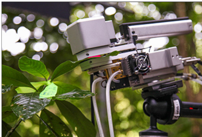
A machine tracks the rate of photosynthesis and carbon dioxide uptake by a leaf. Photo by Gayathri Vaidyanathan.
