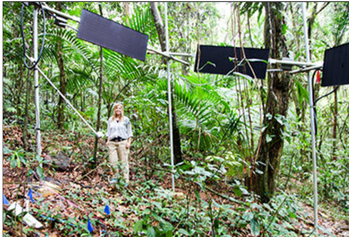
Scientists are warming a patch of forest by 4 degrees Celsius to see how it responds to global warming. A hexagonal metal canopy holds heaters. Photo by Gayathri Vaidyanathan.
